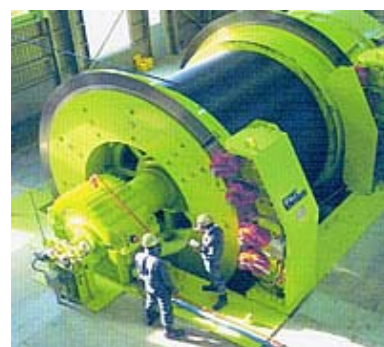
Figure 6: The worldwide longest winding machine for inclined shaft with length of 7,000m. (provided by Kusio Colliery )
